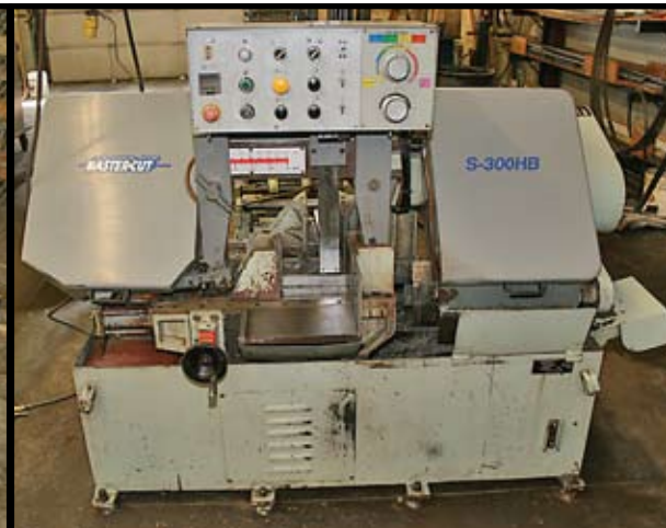
(1994) Master-Cut Model S-300HB Automatic Saw with 11" x 12" capacity, bundle bar clamping and coolant
