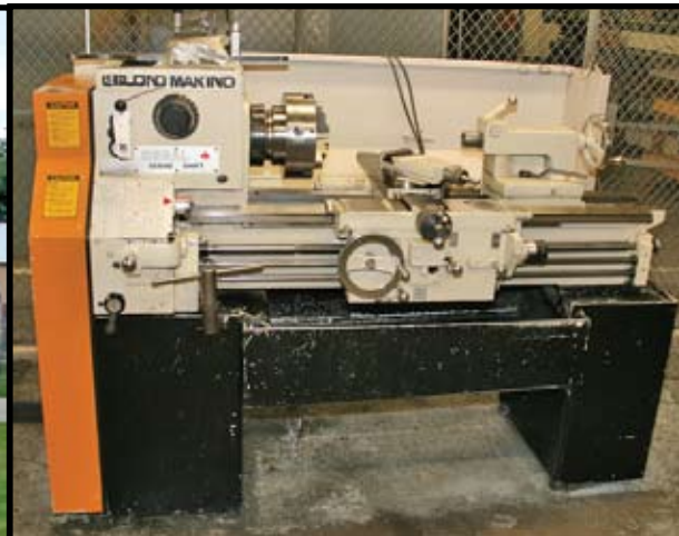
LeBlond Makino 15" x 40" Lathe with Acu-Rite III Digital Readout, tailstock and carriage
