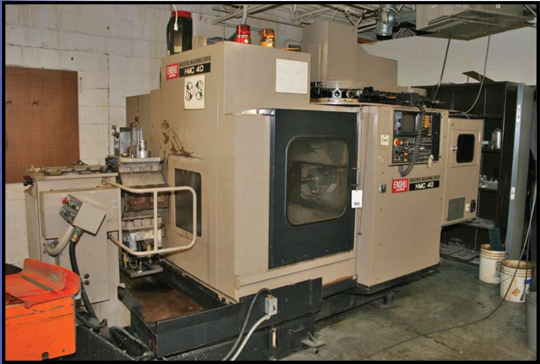
Enshu HMC 40 Pallet Machine with four pallet changer capacity with Fanuc 11m Control
