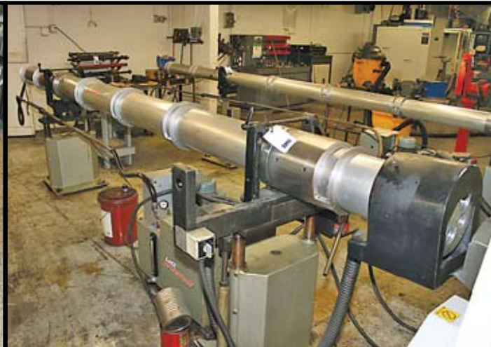
(4) LNS Hydro bar Feeders (Models 6.35 HS-4.8; 6.65 HS-5.2; 6.40 HS-5.2 and 6.32 HS-5.2)
