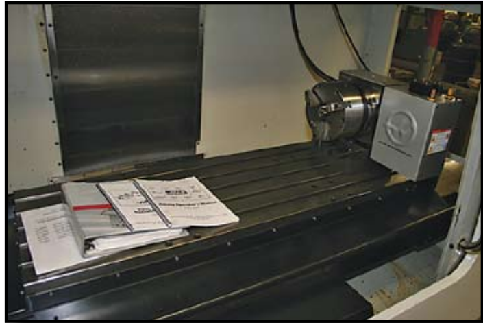
(2005) Haas VF-4B VMC with rotary 4th axis
