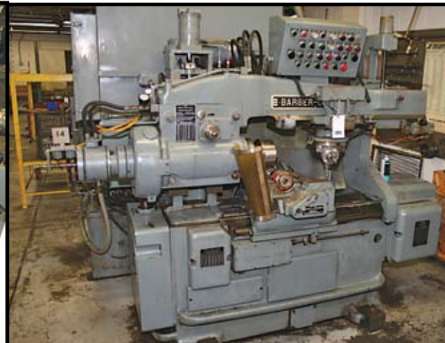
(2) Barber Colman Gear Hobbers with 13" capacity and indexing table
