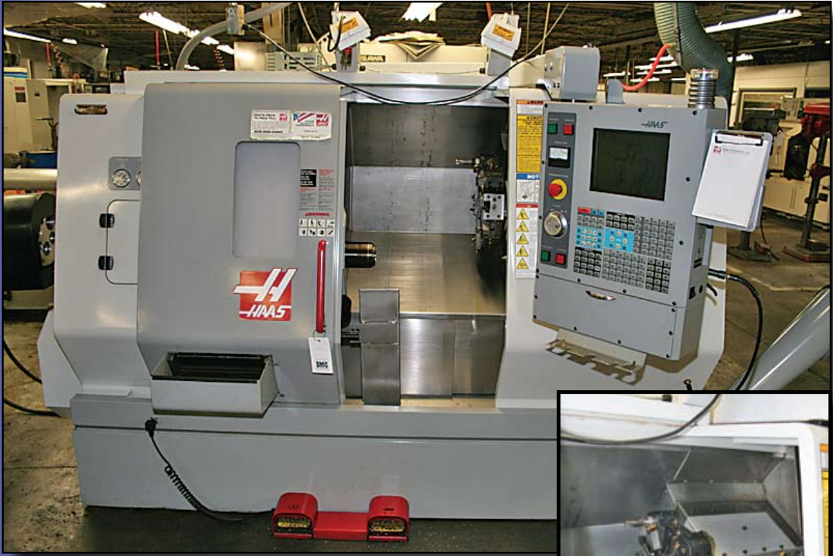
(2004) Haas SL-20C CNC Lathe with parts catcher
