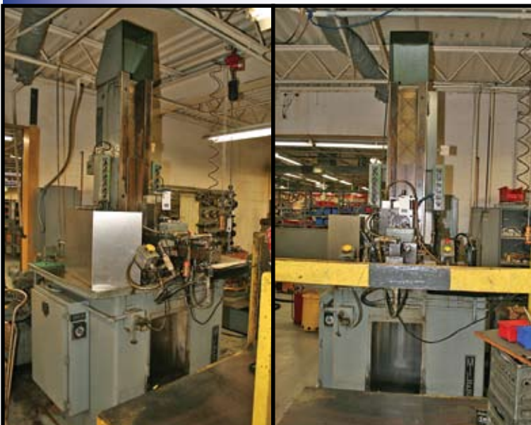
Miles Vertical Broach Model: MBHD121-36-120R with work platform
