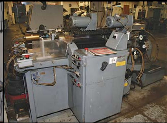
Eldorado Gun drill Model: M75-1071 with dual heads
