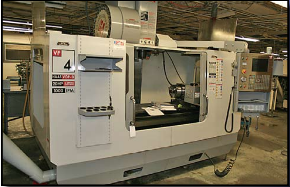
(2005) Haas VF-4B VMC with rotary 4th axis
