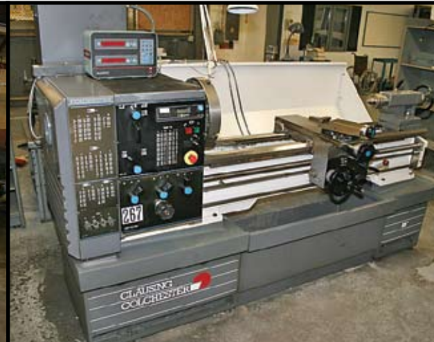
Clausing 15" x 50" with 8" chuck, tailstock and steady rest, faceplates and English Threading
