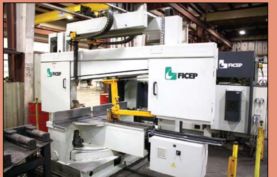
Ficep Beam & Drilling Line Model: 1101ZB, Year: 2006 with 40" wide powered conveyors including (4) 8' conveyors & (5) 5' conveyors and (2) 3' Infeed Conveyors max. thickness that can be drilled - 100mm, max. length 12,000 mm; max. positioning weight 5,400 kg
