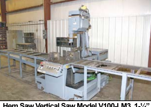
Hem Saw Vertical Saw Model V100-LM3, 1-1/2" Blade, Built-in Coolant Capacity: 18" X 22"
