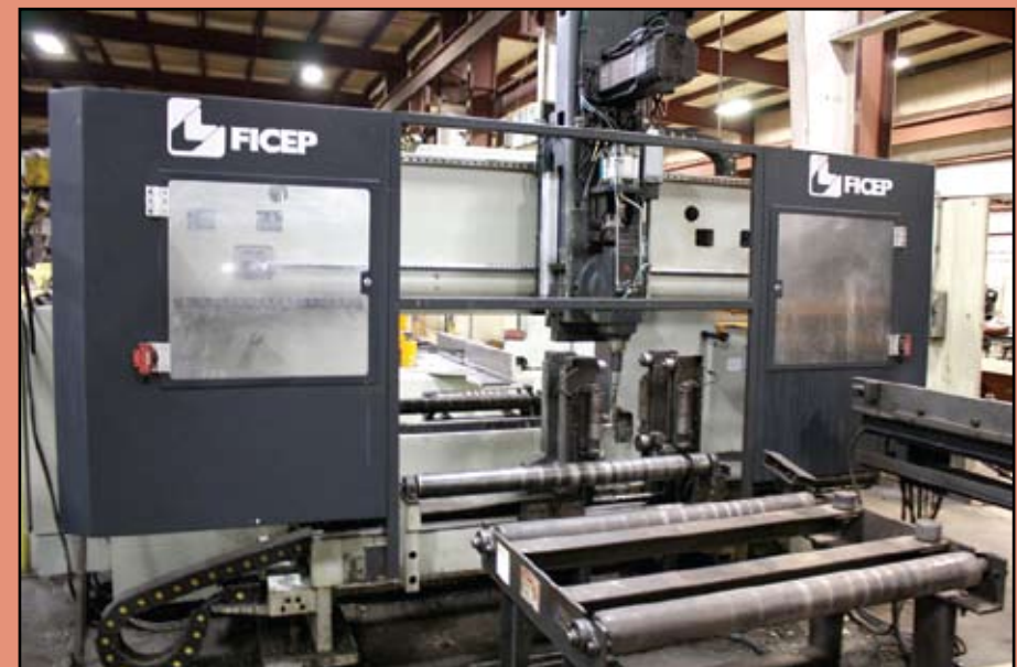
Ficep Beam & Drilling Line Model: 1101ZB, Year: 2006 with 40" wide powered conveyors including (4) 8' conveyors & (5) 5' conveyors and (2) 3' Infeed Conveyors max. thickness that can be drilled - 100mm, max. length 12,000 mm; max. positioning weight 5,400 kg
