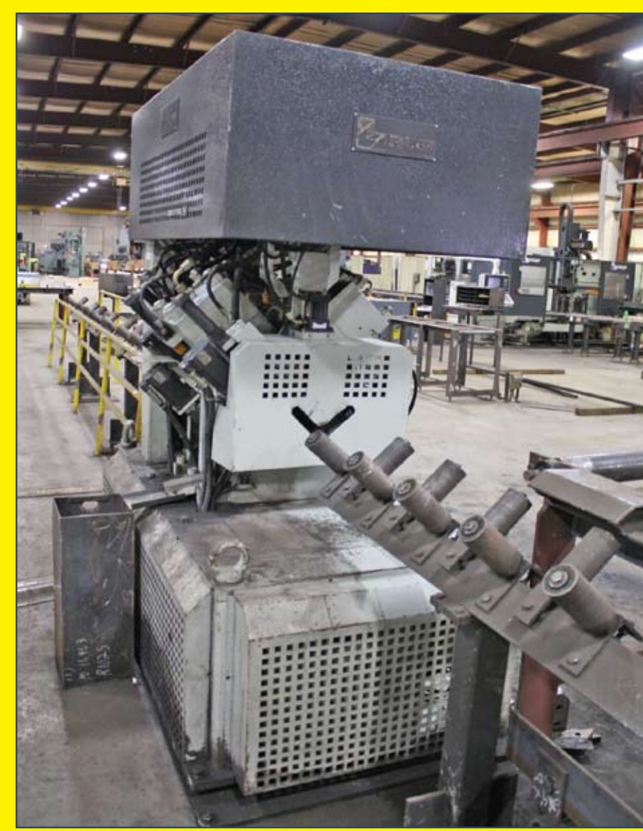
Ficep CNC Angle Line Model: A152, Year 2003. MAXIMUM PUNCHING CAPACITY - TONS; MAXIMUM SHEARING CAPACITY - 200 TONS; CNC AXES -3
