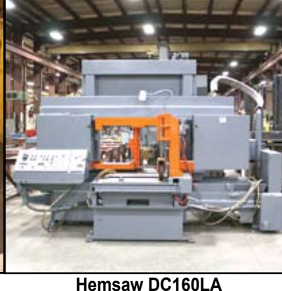
Hemsaw DC160LA Capacity 25" X 30"
