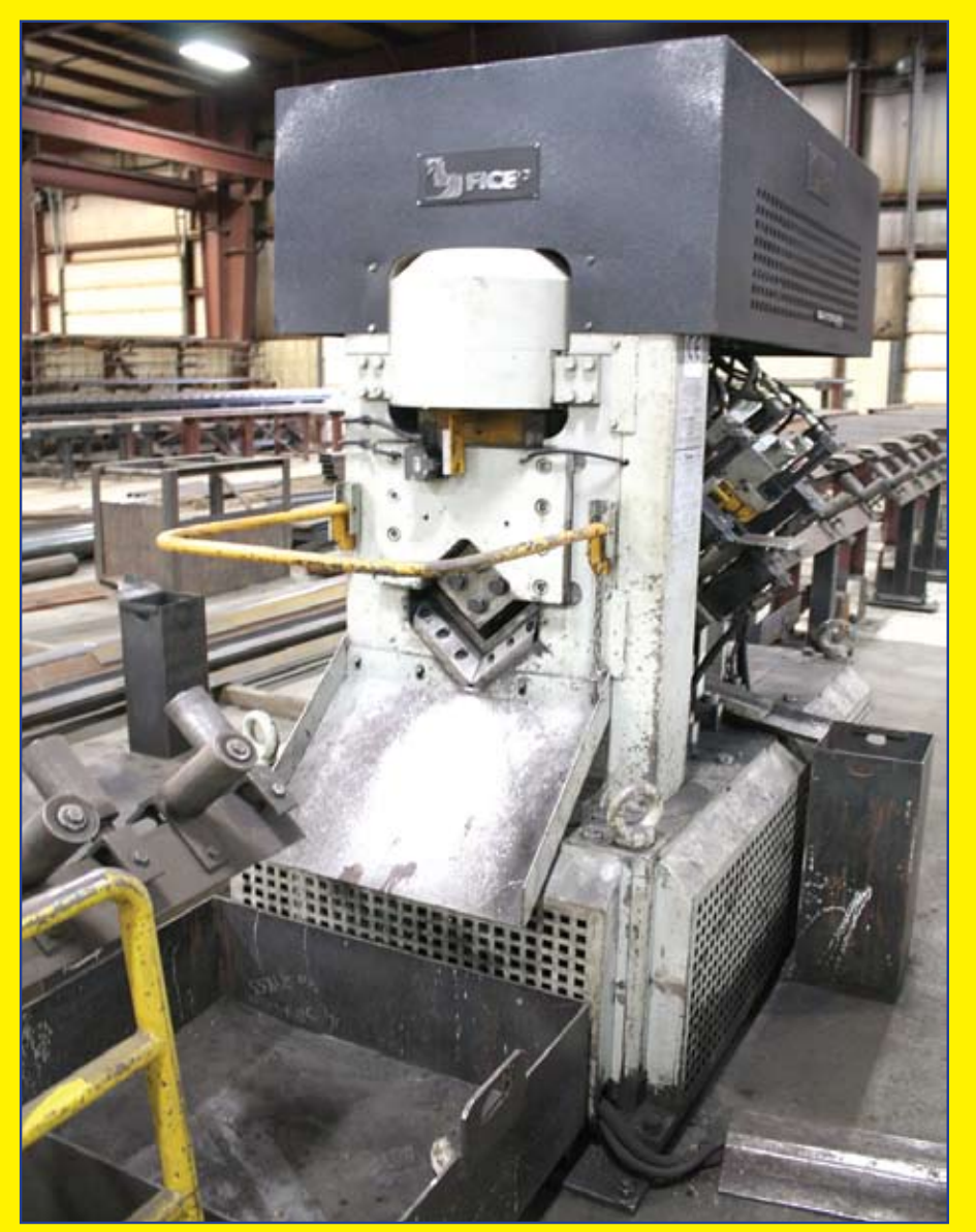
Ficep CNC Angle Line Model: A152, Year 2003. MAXIMUM PUNCHING CAPACITY - TONS; MAXIMUM SHEARING CAPACITY - 200 TONS; CNC AXES -3
