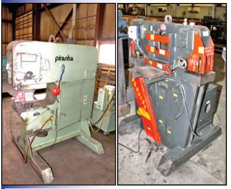
Pirahna 120 Ton Punch Edwards 75 Ton Ironworker
