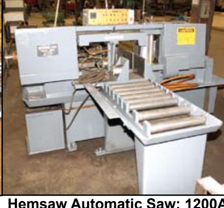
Hemsaw Automatic Saw: 1200A, 24" Stroke Capacity 16" Round
