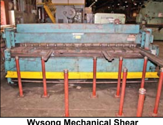
Wysong Mechanical Shear 10" - 10 Gauge
